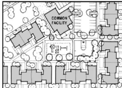
Buildings are configured to form a centralized open space area for children’s outdoor play
