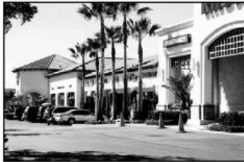
Changes in height, wall plane and volume mitigate the linearity of long buildings and provide an interesting environment
