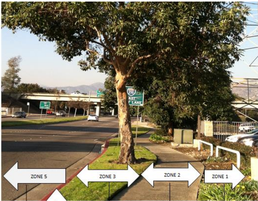
Image of root restriction zones for excavation, trenching, or boring within a tree dripline in a planting strip.
